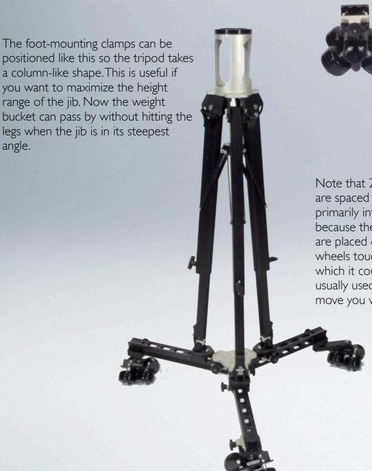
Note that 2 of the 4 wheels per cluster are spaced out differently. These wheels are primarily intended to be used on track. However, because they are spaced out like this, when they are placed directly on the floor, only 2 of the 4 wheels touch the floor. This allows the dolly to roll on the floor which it could not do if all 4 wheels were touching. This feature is usually used simply to reposition the jib. To actually do an in-camera move you would need to be on a very smooth floor.
