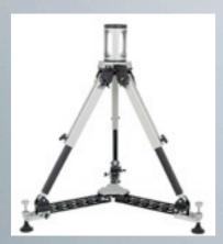
Note: The Explorer Version I Tripod looked like this. It had short legs, clamps for feet, and a large spreader base with leveling feet. It was designed like this to make it a quick change-over to a 3-Leg track dolly by exchanging the leveling feet for dolly wheels. It worked well as the jib/trolley support, but it was slow to set up because the spreader base needed to be assembled, and its short legs made it impractical as an everyday tripod.
