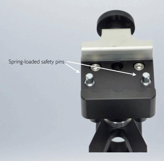
Note that the front and rear assembly clamps have two spring-loaded safety pins. Only one is used. The second is there as a safety so that if you accidentally have the clamp upside down, it will still engage into the safety slot of the rail.
