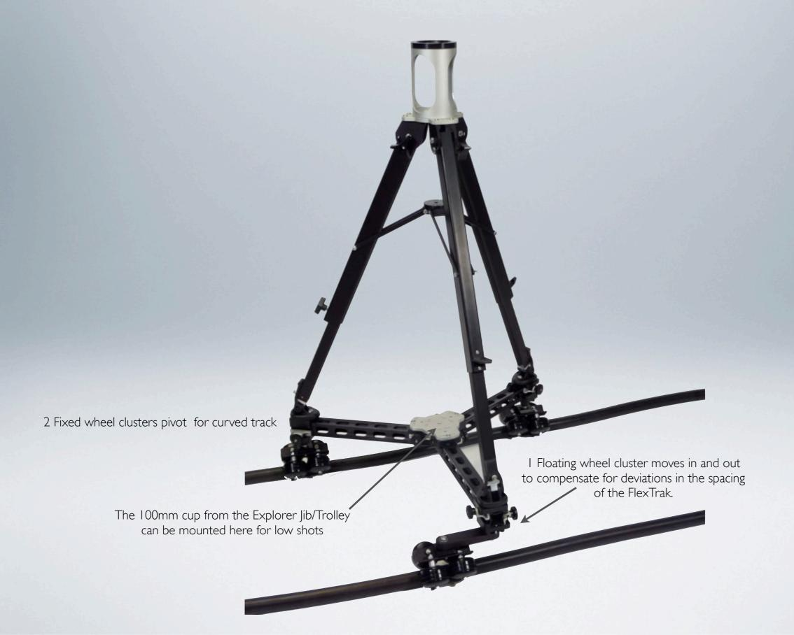
To assemble dolly, clamp the three rails to the center plate, clamp wheels to the end of the rails, and add the three foot-mounting clamps.
