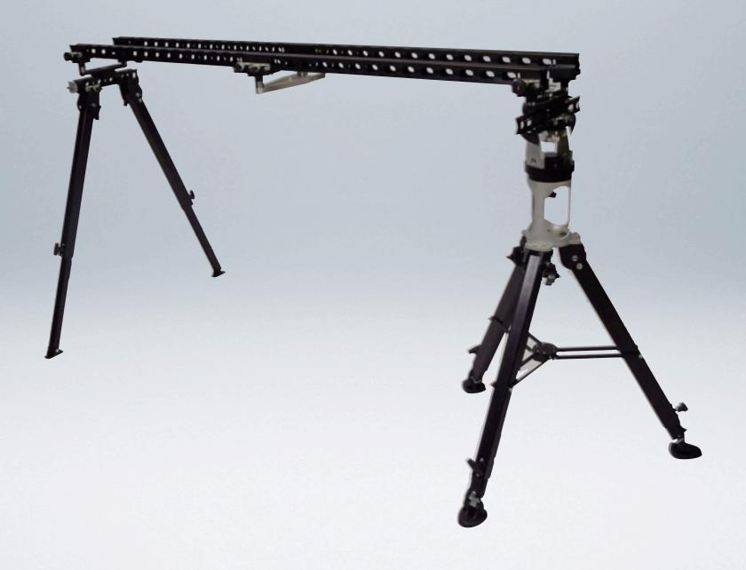
Once knobs are removed, lift out the complete rail assembly as a unit and place it on the ground .
