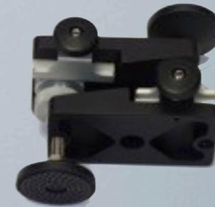
Tighten the clamp knobs to minimize the width of the monopods
