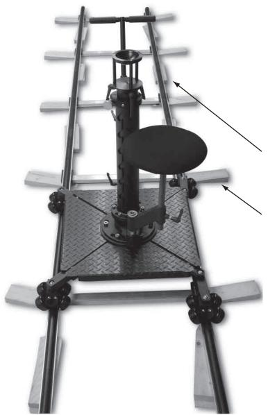
A frame made with our FlexTrak Channels and our new Channel Spreaders can be leveled with traditional dolly track wedges. Because FlexTrak has no seams, leveling does not need to be as precise as it does with traditional track, which greatly reduces set-up time. Simply place the end of each channel into the plastic receptacle on each spreader to create the frame, then position the FlexTrak into the channels.
